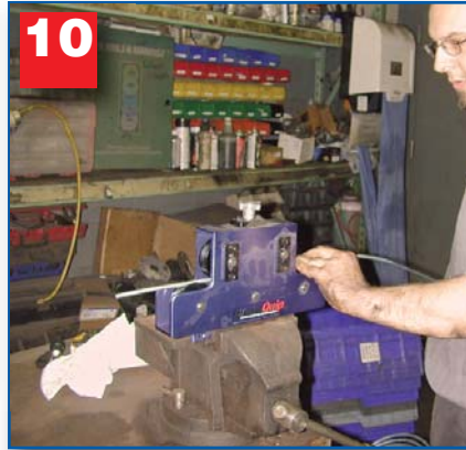
10 Many shops stock rolls of various diameters of brake-line tubing. This makes the work easier with the tools we have for the job. Clamp the straightening tool in a vise and start the rolled line through it.
