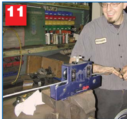
11 Work it back and forth a few times and you will get a straight line of tubing such as this.
