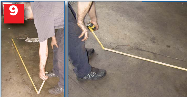
9 We used a tape measure to make sure we could get the length as close as possible to the line that was removed. It's better to cut a little long to make sure you have enough length to form the flared ends.
