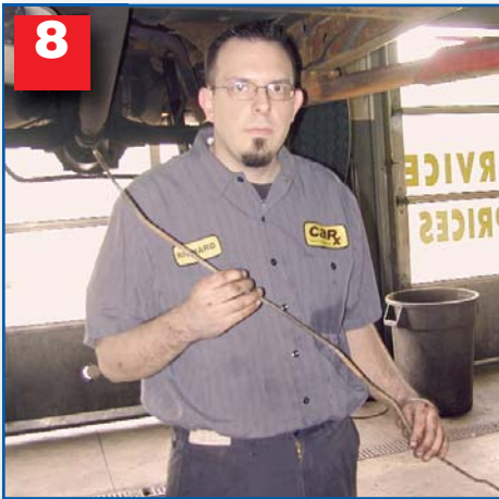
7 Here we've removed the line. Instead of cutting out the sections, it's important to take the line out in one piece so you can measure it. Make sure to retain the original bends.
