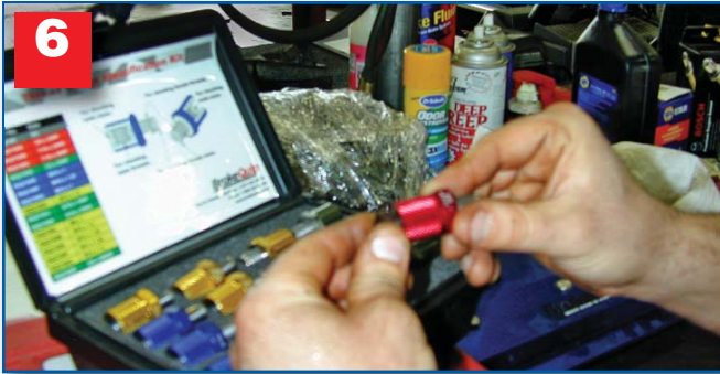
6 With the line removed you can see the size and pitch of the flare nut. Make sure you compare the old nut with the new to make sure you use the same-size nut.
