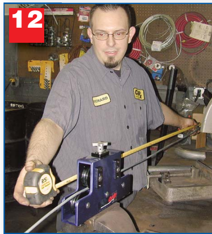
12 Take a measurement to make sure your length is similar to that of the line you removed.
