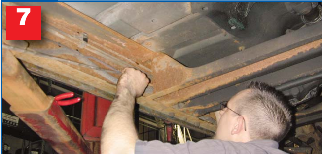
7 Here we've removed the line. Instead of cutting out the sections, it's important to take the line out in one piece so you can measure it. Make sure to retain the original bends.
