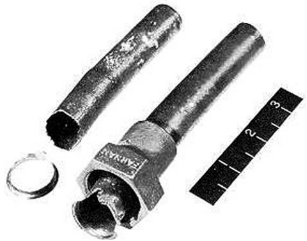
Figure 2: Burst-pressure test results under salt-spray-exposure conditions for 90-10 copper-nickel and steel brake tubing.
