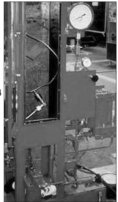
Figure 4. Equipment used to test hydrostatic pressure in brake tube.
