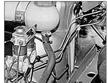
Figure 1. Copper-nickel brake lines running from master cylinder in 1990 Volvo.
